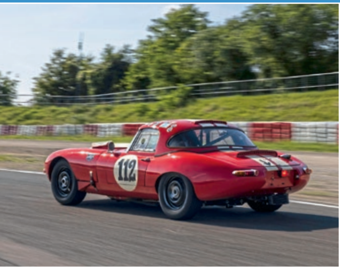
270 hp was sensational in the sixties, resulting in a top speed of nearly 240 km/h. Adapter plates with central locking allow the mounting of steel wheels
